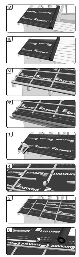
The way the roof membrane is laid as a layer of initial roof covering depends on the roof pitch and the final roof covering material. If the roof pitch is too shallow or too steep, it is recommended to read carefully the covering assembly instruction supplied by the roof covering manufacturer.
